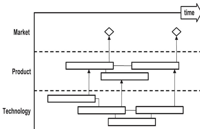
Fig. 1 Generic schematic of technology roadmap [6]
