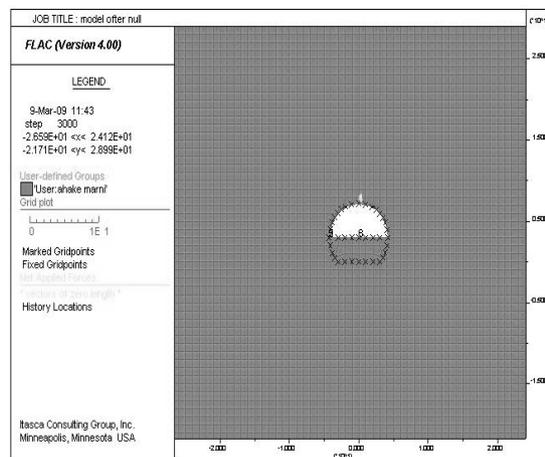
**Fig. 2** The first step of tunnel excavation
