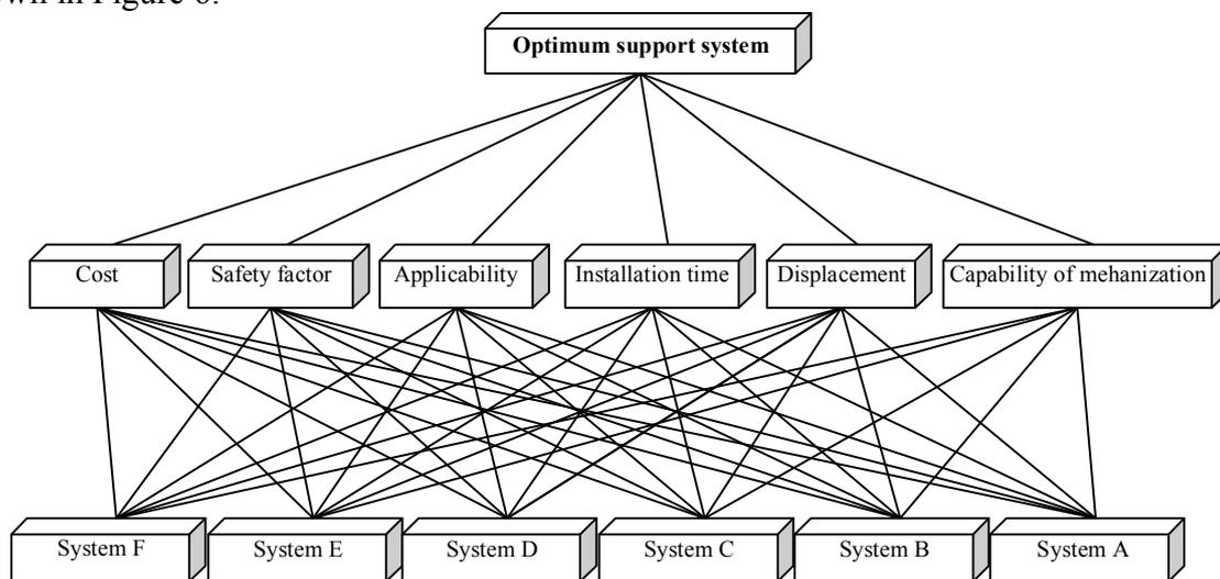
**Fig. 6** Hierarchy design for the tunnel support selection
