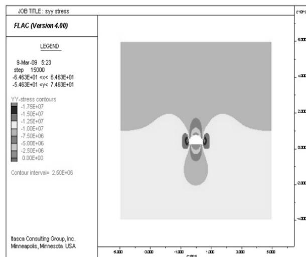
Fig. 5 Stress and displacement around the tunnel at the second phase of excavation
