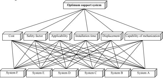
Fig. 6 Hierarchy design for the tunnel support selection
