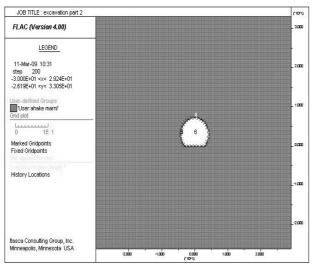
Fig. 3 The second step of tunnel excavation
