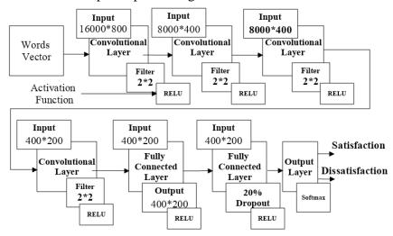
Fig. 2 Structure of the convolutional deep neural network
