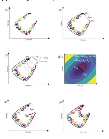
**Fig. 2** Generated output dots (A); initially identified convex boundary (B); new objective function minimized to identify other output dots within circular or elliptical regions (C); elliptical contour plot of the new objective function with R=2 (D); boundary updated with a new  $h_{max}$  value (E); the process successfully identifies concave boundaries (F)
