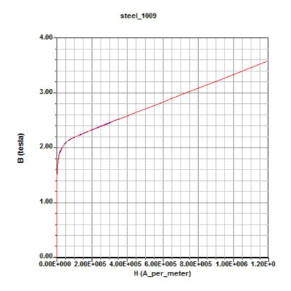
Fig.2 B-H curve of steel used for FEA
