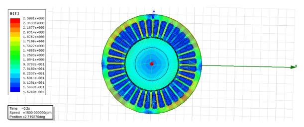
Fig. 10 Flux density distribution
