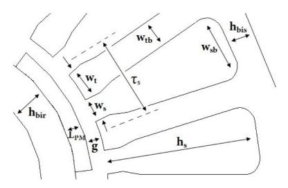
Fig.1 Motor topology showing geometrical definitions
