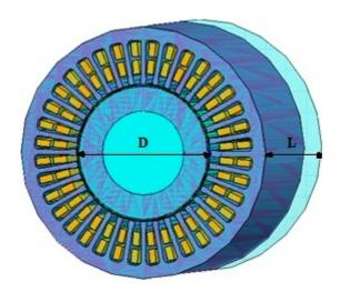
Fig. 3 Motor's main dimensions
