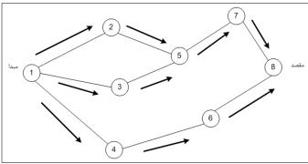
Fig. 2 broadcast for route discovery in AODV
